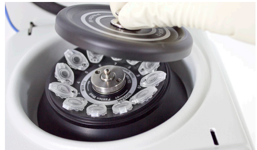
Built-in rotor MSR-12 and a protection lid
